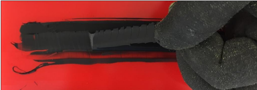
Figure 20: Peel adhesion test: pulling the bead apart, result: 100% cohesive failure
