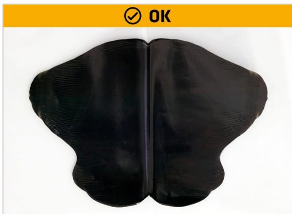
Figure 7: Unfold the foil - Positive test = ideal mixing
