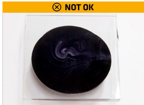
Figure 4: Negative test = inadequate mixing
