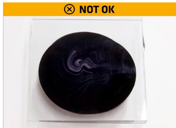
Figure 4: Negative test = inadequate mixing
