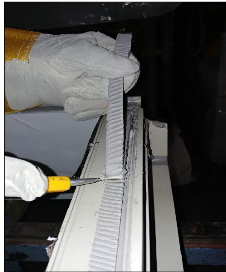
Figure 37: Testing joint adhesion along the whole frame – Good adhesion.
