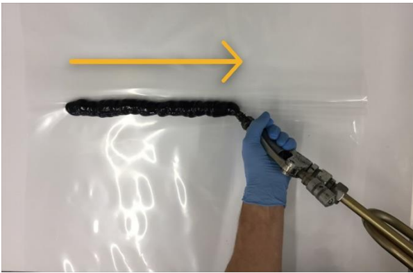
Figure 5: Apply the bead in the fold direction
