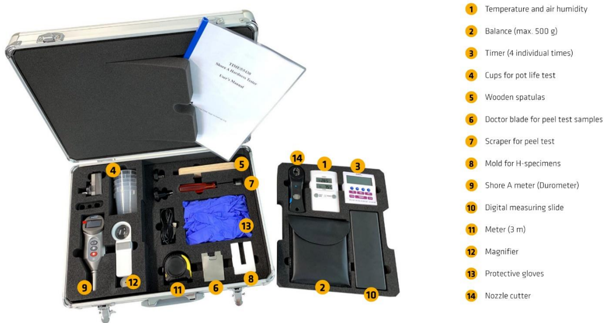
Figure 2: Pocket lab / Lab case for quality control
